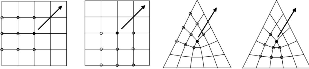
Figure 17: Stencils for  $x$  and  $y$  gradient components in 2D. Black arrow shows direction of velocity at bolded point. Left two meshes show points used to construct stencils for  $x$  and  $y$  derivatives respectively. Right two meshes show points used to construct stencils for  $x$  and  $y$  at an extraordinary face.
