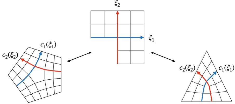
Figure 8: Local three quadrant parametrisation around extraordinary face.
