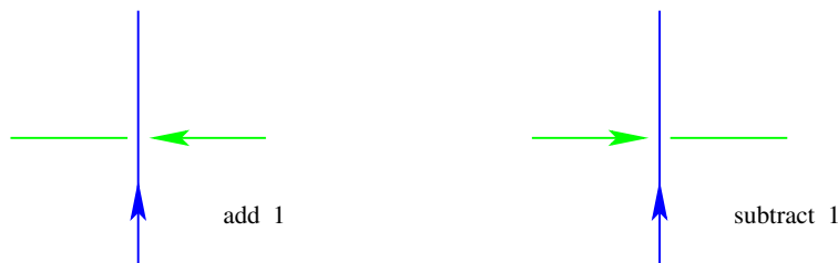
Figure 3: At each crossing add 1 when the underpass crosses leftwards and subtract 1 when it crosses rightwards.
