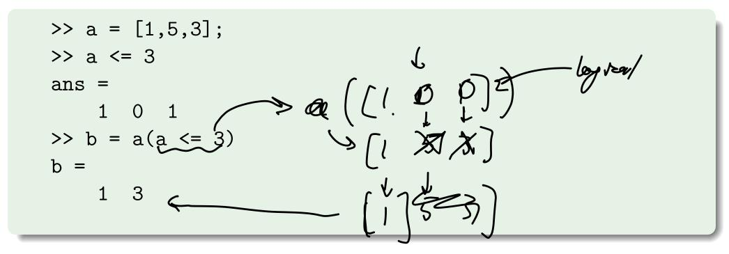
The last command selects all elements in the vector a that are less than or equal to 3.
