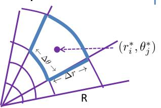
In this new coordinate system, we need to figure out the area of the curved box
