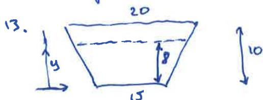
Taking coordinate  $y=0$  at bottom of dam, the width of the dam at height  $y$  is  $15 + y/2$ , and the water
