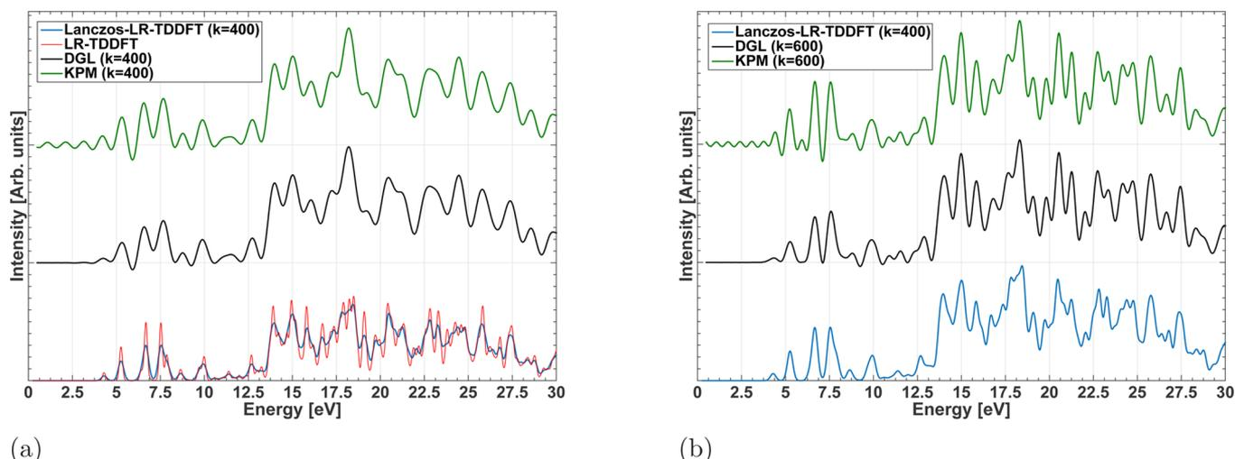
**Figure 6.** Comparison of simulated absorption spectra of TFBA calculated by LR-TDDFT, Lanczos-LR-TDDFT, KPM, and DGL. The FCA was used. (a)  $k = 400$  (b)  $k = 400$  for the Lanczos-LR-TDDFT and  $k = 600$  for KPM and DGL.
