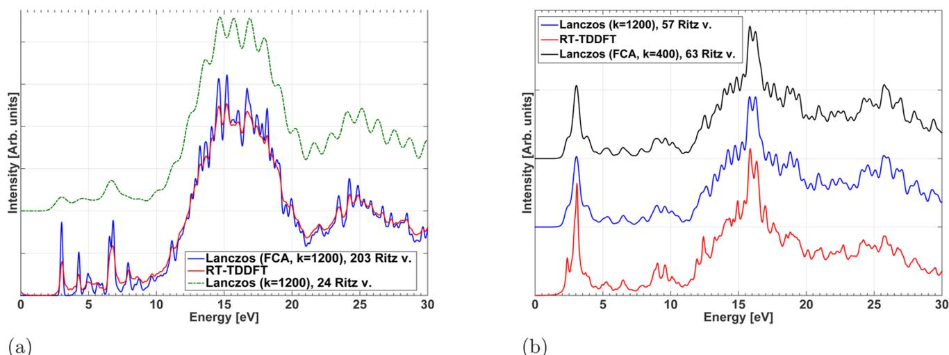
**Figure 5.** Comparison of simulated absorption spectra of F2N12S calculated by RT- and Lanczos-LR-TDDFT with and without FCA. Comparison of simulated absorption spectra of P3B2 calculated by RT and Lanczos-LR-TDDFT. The number of Ritz values in the displayed interval is 57 for  $k = 1200$  or 63 for  $k = 400$  while FCA is used.
