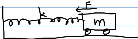
Let  $x$  be the position of the cart, relative to rest length, and  $x'$  its velocity. Newton's 2nd law is the differential equation  $F = mx''$ .  $x''$  is the acceleration of the cart,  $F$  the force applied to it. Hooke's law for springs is  $F = -kx$
