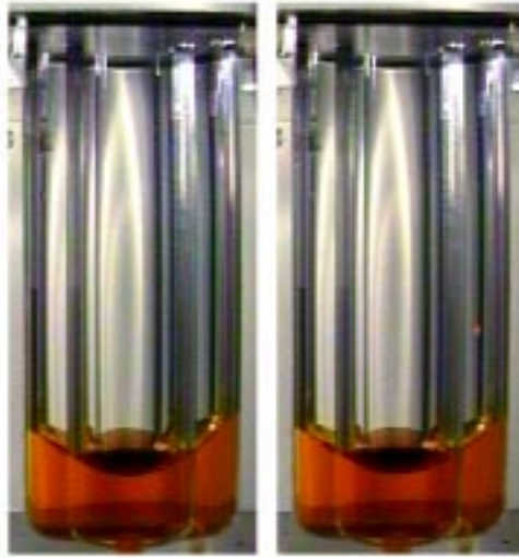
Figures 7a–b. Static interface shapes for ICE-P1 ( 20^\circ/26^\circ ) vessel. 7a (left): after completion of fill; 7b (right): after disturbances by crew member.
