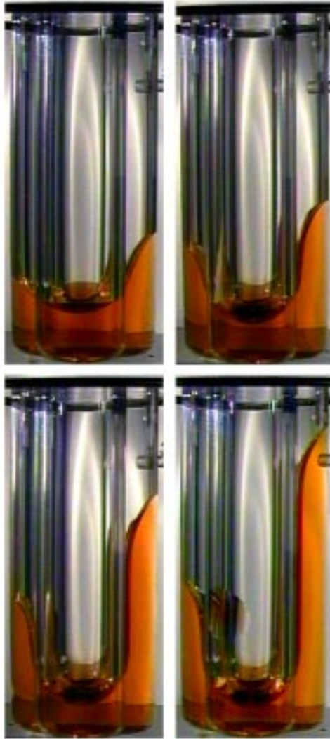
Figures 9a–d. Static interface shapes for ICE-P3 ( 38^\circ/44^\circ ) vessel. 9a (upper left): after completion of fill; 9b (upper right), 9c (lower left), and 9d (lower right) after successive disturbances by crew member.
