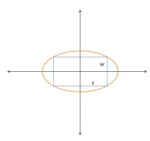
The equation we wish to maximize is A = (2w)(2z). Note first that the ellipse above has width a along the x-axis and height b along the y-axis. To eliminate either w or z, we solve the equation of the ellipse for its positive component:
