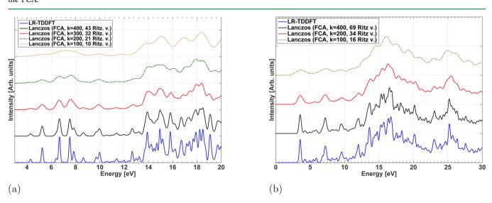
Figure 4. Resolution improvement with respect to the number of Lanczos iterations k for (a) TFBA (b) HBDMI.
