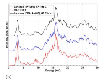
**Figure 5.** Comparison of simulated absorption spectra of F2N12S calculated by RT- and Lanczos-LR-TDDFT with and without FCA. Comparison of simulated absorption spectra of P3B2 calculated by RT and Lanczos-LR-TDDFT. The number of Ritz values in the displayed interval is 57 for k = 1200 or 63 for k = 400 while FCA is used.
