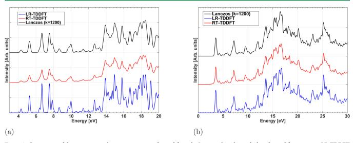
Figure 2. Comparison of the approximate absorption spectrum obtained from the Lanczos algorithm with that obtained from an exact LR-TDDFT calculation and RT-TDDFT calculation for (a) TFBA (b) HBDMI.
