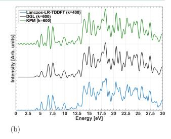
Figure 6. Comparison of simulated absorption spectra of TFBA calculated by LR-TDDFT, Lanczos-LR-TDDFT, KPM, and DGL. The FCA was used. (a) k = 400 (b) k = 400 for the Lanczos-LR-TDDFT and k = 600 for KPM and DGL.
