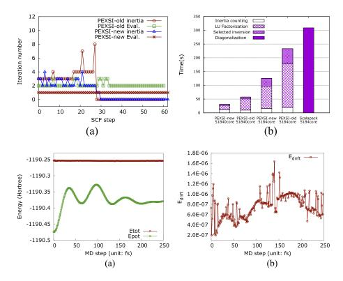
FIG. 6. Comparison of the performance of PEXSI-new and PEXSI-old, and diagonalization for the GRN 6480 system. (a) Number of inertia counting step and evaluation of the Fermi operator steps. (b) The timing for PEXSI-new, PEXSI-old, and diagonalization per SCF step.
