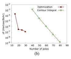
FIG. 4. Error of the (a) energy and (b) force of the PEXSI method with respect to the number of poles for the graphene 180 system.
