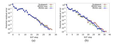
FIG. 5. SCF convergence with ScaLA-PACK and PEXSI-old and PEXSI-new along the SCF steps for (a) PNR 180 and (b) GRN 180 systems.
