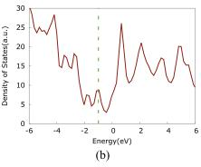
FIG. 3. The total densities of states (DOS) of (a) PNR and (b) GRN 180 atoms, respectively. The fermi levels are marked by the green dashed line.
