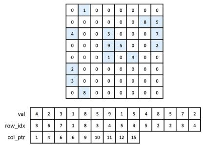
**Fig. 4.** An 8 × 8 matrix stored in (a) dense storage format versus in (b) compressed sparse column (CSC) storage format. In the CSC format, only the values of the non-zero elements, indicated in blue in (a), are stored in the "val" array. The row indexes of the non-zero elements are stored in the "row\_idx" array. The "col\_ptr" array stores the starting points of the matrix columns.
