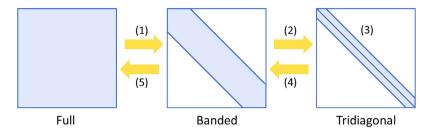
**Fig. 1.** Five computational steps of the ELPA eigensolver with two-stage tridiagonalization. (1) Reduction of the full matrix to a banded form. (2) Reduction of the banded matrix to a tridiagonal form. (3) Solution of the eigenvectors of the tridiagonal system. (4) Back-transformation of the eigenvectors to the banded form. (5) Back-transformation of the eigenvectors to the original full form. This figure is redesigned based on Fig. 1 in Ref. [15].
