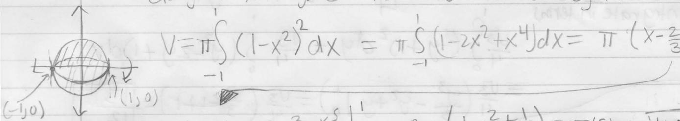
$$V = \pi \int_{-1}^1 (1-x^2)^2 dx = \pi \int_{-1}^1 (1-2x^2+x^4) dx = \pi \left( x - \frac{2}{3}x^3 + \frac{x^5}{5} \right) \Big|_{-1}^1$$
