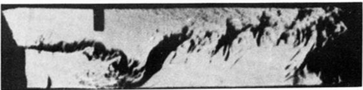
FIGURE 1. Photographic schlieren records of turbulent combustion stabilized behind a step, in a propane-air mixture at an equivalence ratio of 0.57, entering the channel at u'_{\infty} = 13.6 \text{ m s}^{-1} ( R = 22 \times 10^4 ) while T_{\infty} = 295 \text{ K} : (a) growth of a large eddy under the influence of recirculation (time interval between frames: 1.22 ms); (b) 'steady-state' propagation of a large-scale ('coherent') structure (time interval between frames: 1.16 ms).
