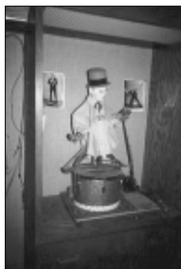
Shannon’s juggling machine, constructed sometime around 1983. Built mostly from pieces of an erector set and dressed to look like W. C. Fields, the machine bounce juggles three small metal balls in a cascade off a drum.
